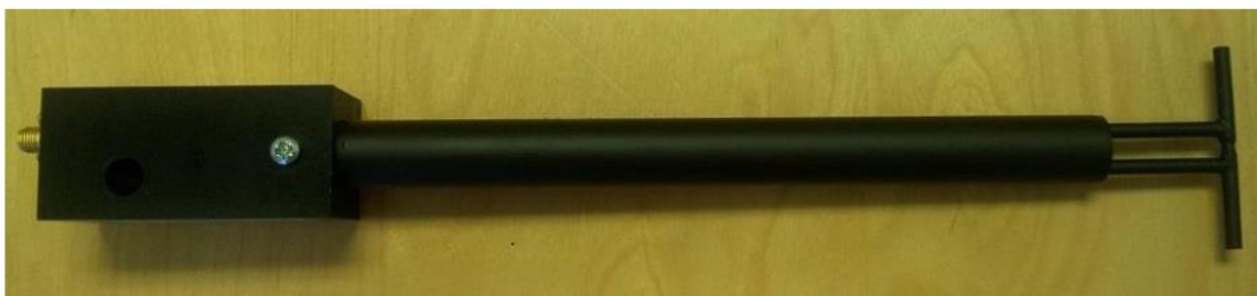
Figure 1 – MVG COMOSAR Validation Dipole
